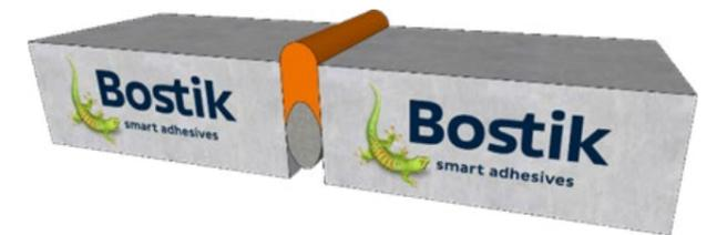
Example 2: Expansion of the building materials due to temperature absorption. Result is that the joint in between the adjacent building materials will be 'smaller'.
