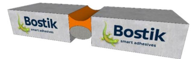
Example 3: Contraction of the building materials due to temperature remittance. Result is that the joint in between of the adjacent building materials will be 'wider'.
